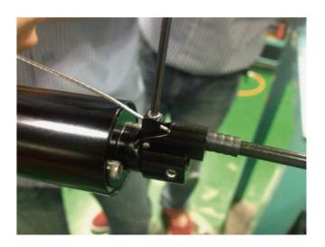
10) PULL SHIFTER CABLE TAUT TO REMOVE ALL SLACK AND TIGHTEN THE CABLE FIXING BOLT. THIS SET SCREW MUST BE VERY TIGHT OR CABLE CAN PULL OUT.
