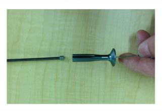
2) INSTALL SHIFTER CABLE THROUGH ACTIVATION LEVER AND INSTALL THE SET SCREW INTO THE END OF THE LEVER TO HOLD THE CABLE IN PLACE.
