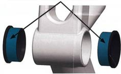
3 Press each cup individually using the headset press. Cups must be flush to the frame before installing the BB.
