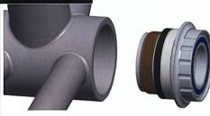
7 Start threading the Drive Cup inCLOCK-WISE with your Shimano BB tool. As it threads in, you will feel friction build as the compression o-ring expands against the frame. This is normal. Grab your 2nd BB tool at this point.
