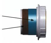
4 Apply thin coating of GREASE to the outside of the Compression O-ring and Compression Sleeve.
